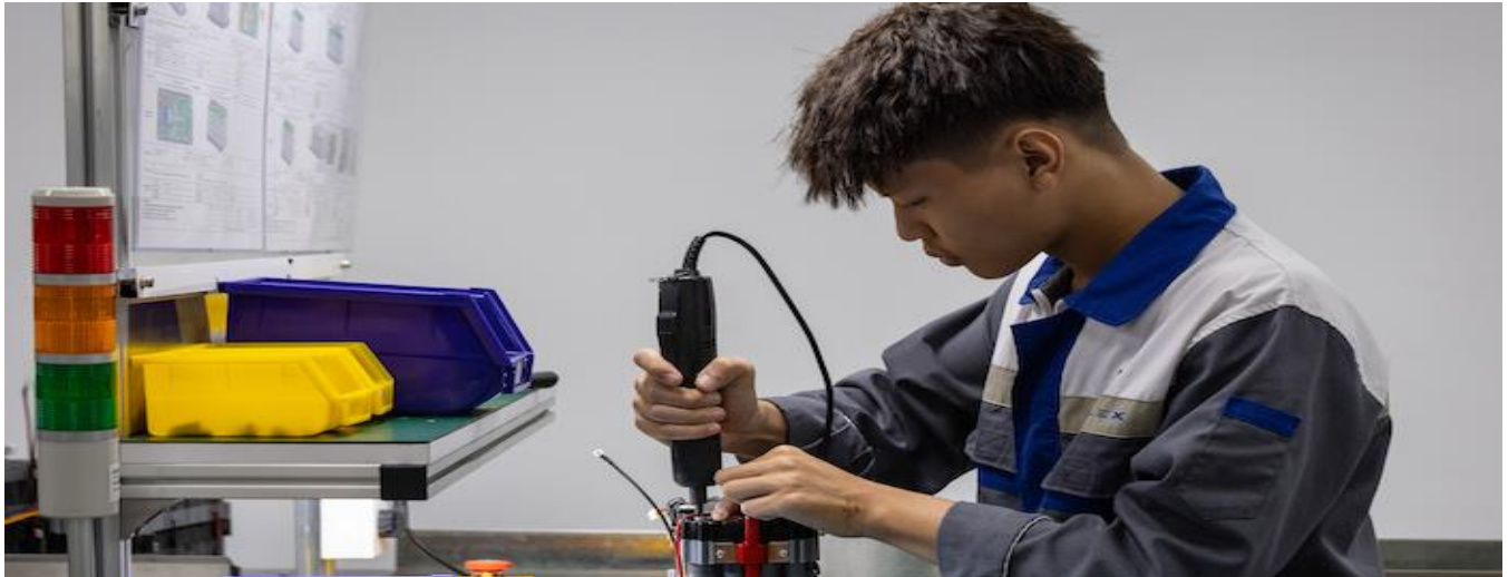
A Vietnamese worker at a smart electric vehicle factory outside Hanoi attaches thermal sensors and charging cables to a battery pack. (Photo: Chris Trinh via Getty)
